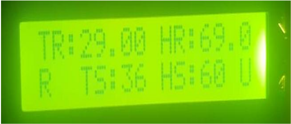
Plate3.1: Temperature and humidity sensor reading on LCD
